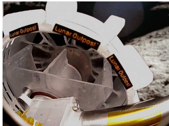
Figure 2: Resource Collection Hopper; View from MAPP Wheel Observation Camera
